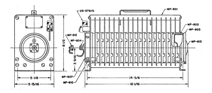
Figure 5-1. Parts Illustration, DA-412A/U
